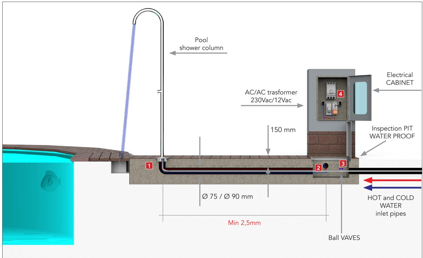
The Bossini column with internal heating system requires that installation be carried out by qualified personnel for the hydraulic and electrical parts, in compliance with current national standards.
